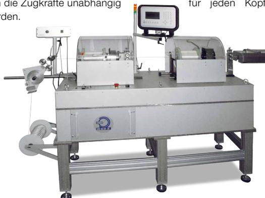
The spiral winding machine KWM-Executive-DK with two winding heads enables to wind two winding materials to one carrier after each other in only one winding process. Both heads are controlled independent of each other from one controller. This allows for example to program different pitches, rotation direction as well brake tension for each head.
