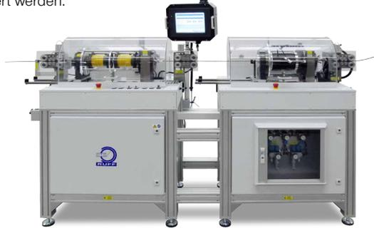
This special spiral winding machine has two independent programmable winding heads, which suits excellent for winding applications of one carrier with two different winding materials to be wound in one process. Further more, with the double spool unit, two wires can be wound simultaneously and the second winding head can be programmed in the same or in the opposite winding direction, according the requirement.
