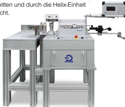
This machine has a heated nozzle with stepless adjustable regulator for the temperature. It is for example for heated bondable wires, when the winding wire will be fixed in the bondable enamel of the carrier. At this special machine, after the winding: the products will be cut to the required length and further it will be wound by the helix unit in a spiral shape.
