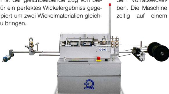
The here shown KWM-EXECUTIVE-2B machine has a double spool unit with two independent programmable brakes for the winding materials. Herewith both spools have continuously the same tension during the process for a perfect winding result. The machine is designed for simultaneous winding of two winding materials to one carrier.
